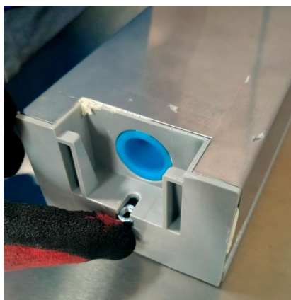
Photo 10: Assembling position of the spacers, with nuts and screws.
