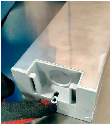
Photo 10: Assembling position of the spacers, with nuts and screws.
