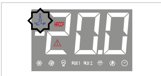
The flashing icon indicates the activation of the OVER COOLING function
