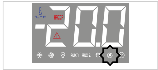
This LED indicates the activation of the ENERGY SAVING function
