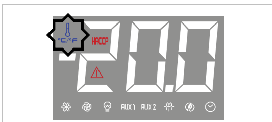
The flashing icon indicates the activation of the OVER COOLING function
