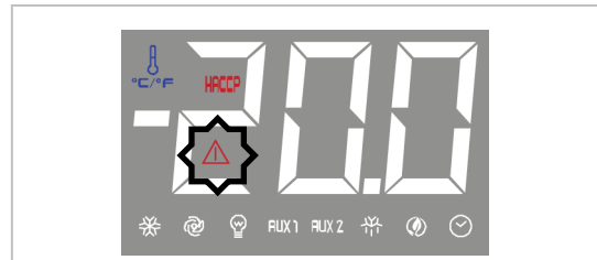
The flashing LED calls for cleaning the condenser filter
