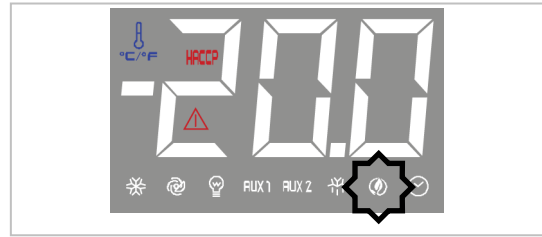
This LED indicates the activation of the ENERGY SAVING function
