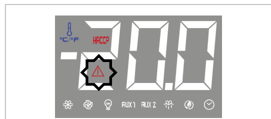
The flashing LED calls for cleaning the condenser filter
