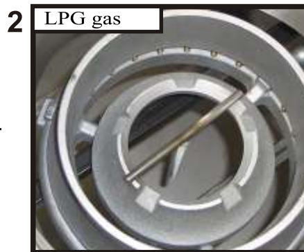
Perforated plate for decreasing the supply of air.
