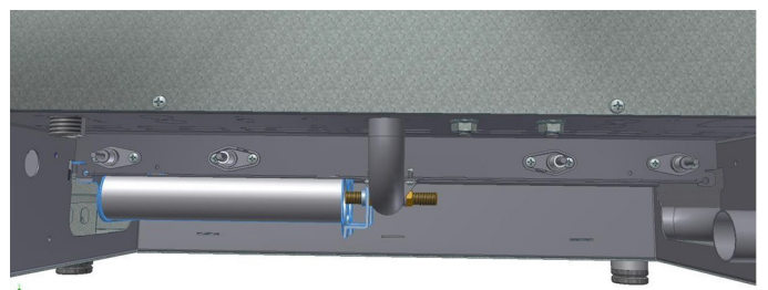
Remove the left burner and the right one.
