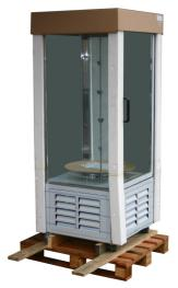
Tilt the cooling display slightly and slide wooden planks under the wheels so that the wheels are aligned with the slope. The planks must protrude as far as possible from the pallet.
